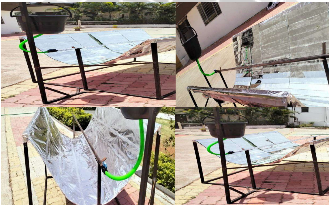
Figure 5.2: Compound parabolic solar collectors with receiver tube
